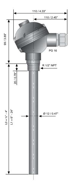
Industrial probes and boards are base on : Ro = 100 Ohms R 100°C = 138,5 Ohms
