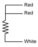
2 / 3 wires setting for industrial applications. This setting limits the effect of lines resistances
